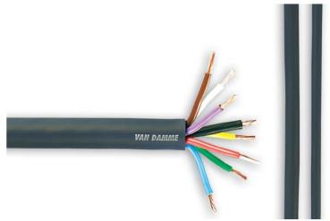
Van Damme Ecoflex Install Grade Speaker Cable LSZH is a Low Smoke Zero Halogen insulated and jacketed cable range. it is specifically designed for installation in public buildings and other areas where LSZH materials are specified such as new-build housing and marine installations. From 2 x 0.75mm for 100V line to 8 x 2.5mm for low impedance systems most speaker applications are well catered for.
