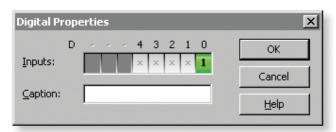
The above pattern will test if, for example, a push switch on digital input D0 is on (pressed). You can see below how to light the green LED on output Q0 whenever the switch is pressed:
