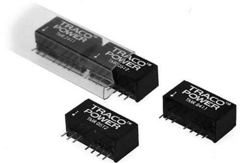
The TMR series is a range of miniature regulated 2 Watt DC/DC- converters in a SIL-package. Requiring only 2cm<sup>2</sup> board space they provide a state of art functionality. Wide 2:1 Input voltage range, 1000 VDC isolation voltage, external on/off control and a temperature range of -40°C – 75°C with no derating makes this converter suitable for many applications in telecommunication, control units and industrial equipments.
