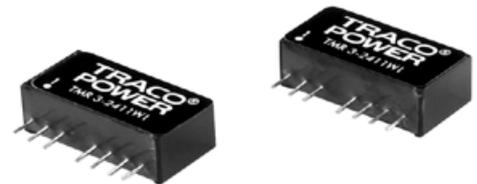
The TMR-3WI series is a new family of isolated 3W DC/DC converters with regulated output, featuring ultra-wide 4:1 input voltage range. The product comes in an ultra-compact SIP plastic package with a small footprint occupying only 2.0 cm<sup>2</sup> (0.3 square in.) of board space. An excellent efficiency allows  $-40^{\circ}$  to  $+85^{\circ}\text{C}$  operation temperatures.
