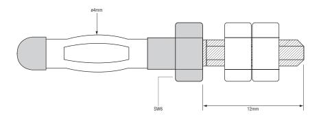
A 4mm plug which can be mounted to printed circuit boards or chassis which mates directly to 4mm sockets.
