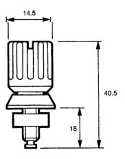
30A Terminal Posts with 4mm top & cross hole. Rugged construction with knurled top which has integral brass threaded insert to enable a secure fixing to any wires in the cross hole. Available with nickel or gold plated contacts and two lengths of rear stud.
