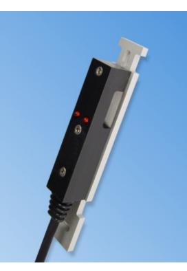
The model with attached tubular sensor can be directly mounted on the inlet of the cooling panels with minimum fitment expenses. The sensor with aluminium profile is fitted on the tube and fixed with the enclosed stainless steel clip. The wiring expenses are also very less. The device is provided with a mains lead and plug, which is only to be connected.
