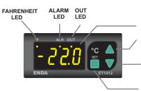
Displayed process value in the run mode, parameter name or value in programming mode.
