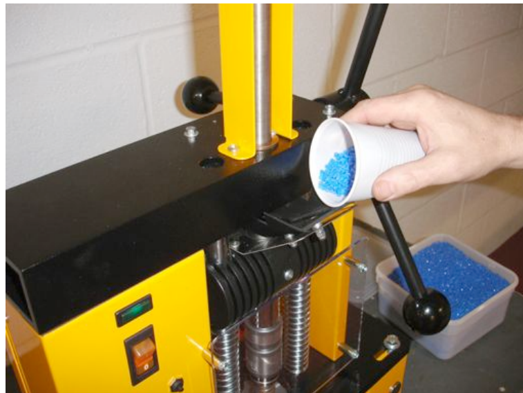
Feeding granules in to the hopper
