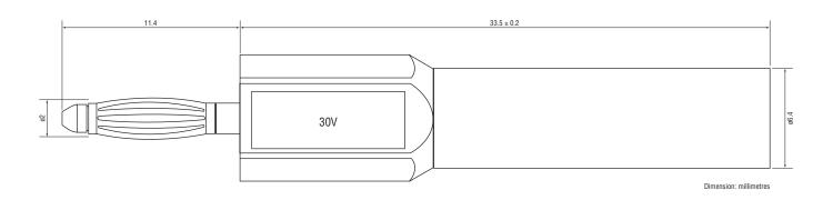
These adaptors convert a 4mm straight plug to a 2mm banana plug. They have a nickel plated brass spring and are housed in ABS.
