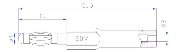
These adaptors convert a 2mm straight plug to a 4mm banana plug. They have a nickel plated brass spring and are housed in ABS.
