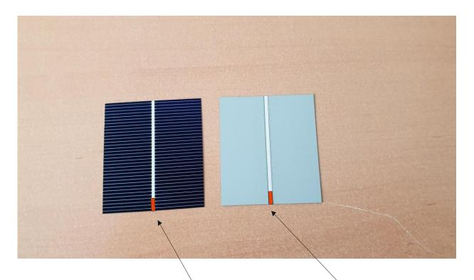
Please solder the cables on the red marked points. On the blue side there is "-" On the grey side "+"
