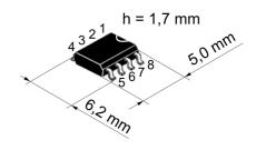
SO8 Housing (150 mil, Standard SMT Technology, SOIC-8) as per IEC 191-2Q: Type 076E35 B
