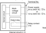
Note: The emitter of the thru-beam type sensor has only two terminals for power supply (terminal No. 1) and 2).
