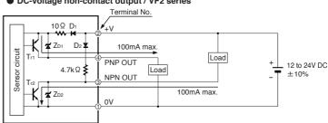
Internal circuit -- 6 →Users' circuit Note: The emitter of the thru-beam type sensor has only two terminals for power supply (terminal No. 1) and 2).
