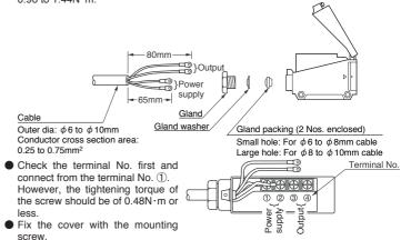
However, the tightening torque of the screw should be of 0.48 to 0.76N·m. Dimensions of the suitable crimp terminals
