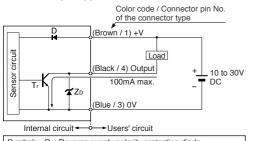
$Symbols...D : Reverse supply polarity protection diode \\ Z_{\rm D} : Surge absorption zener diode$
