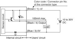
Symbols...D: Reverse supply polarity protection diode Z<sub>D</sub>: Surge absorption zener diode Tr: PNP output transistor
