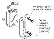
Care must be taken regarding the sensor mounting direction with respect to the object's direction of movement.
