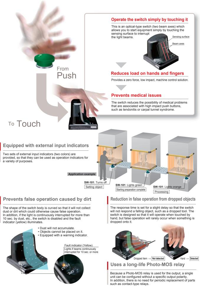
A switch that pursues the prevention requirement for malfunctioning as required by ISO 13851 (JIS B 9712) two-hand control devices
