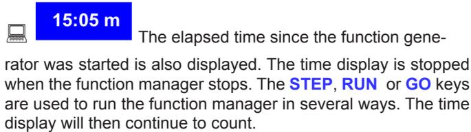
The elapsed time since the function generator was started is also displayed. The time display is stopped when the function manager stops. The **STEP**, **RUN** or **GO** keys are used to run the function manager in several ways. The time display will then continue to count.
