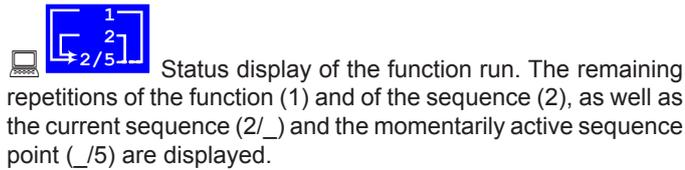
Status display of the function run. The remaining repetitions of the function (1) and of the sequence (2), as well as the current sequence (2/\_ ) and the momentarily active sequence point (\_/5) are displayed.
