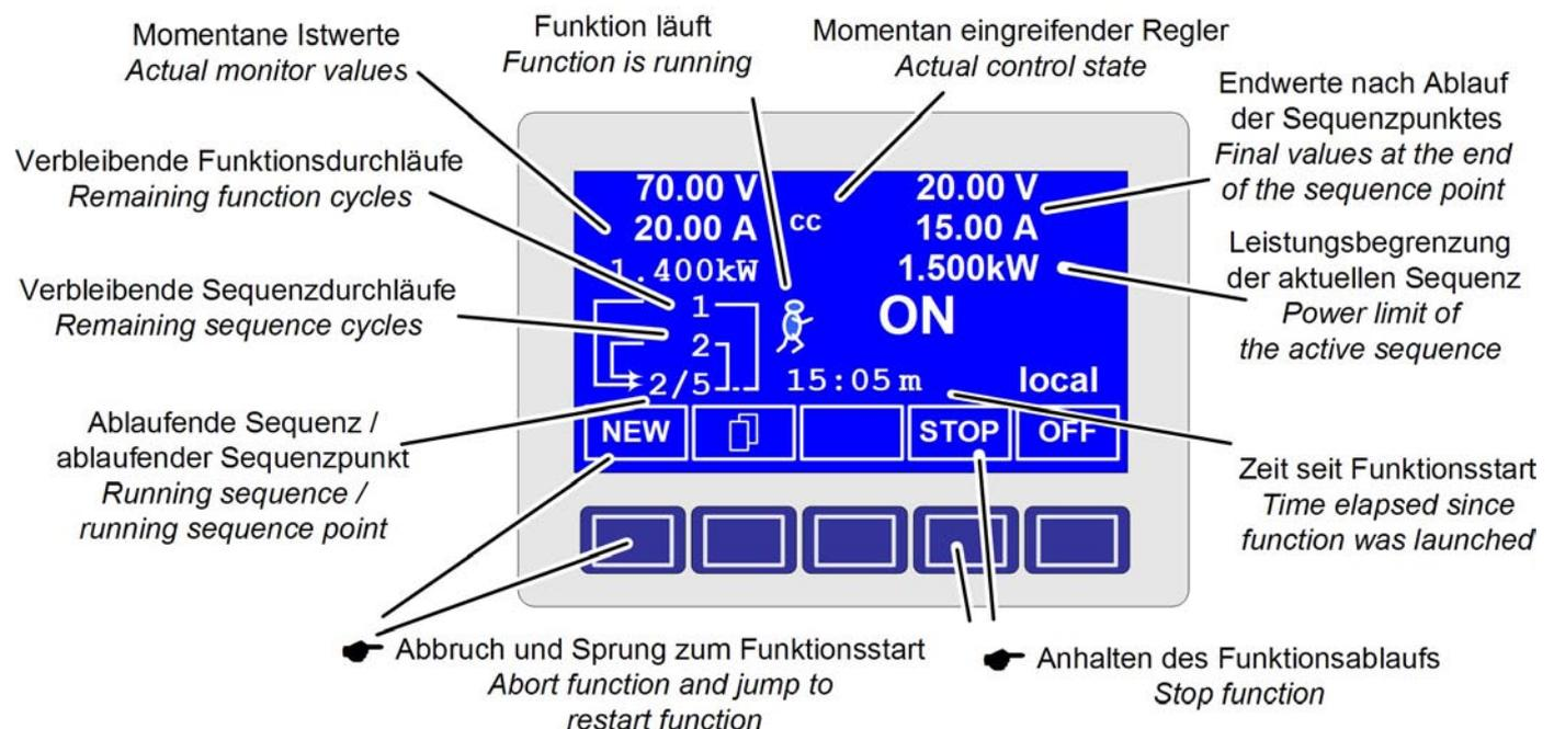
**Function layout** = the configurations in the function layout are used by the function manager to set the operation (U/I/P or U/I/R) mode for the power supply. Furthermore, the repetition rate of the function and the arbitrary order of the sequences are set here. In dependency of the function layout the function manager processes the next sequence after the previous one has been processed and uses the settings from the sequence control of the next sequence.
