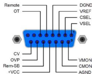
**Attention! Never connect grounds of the analogue interface to minus (negative) output of an external control application (PLC, for example), if that control application is otherwise connected to the negative power supply output (ground loop). Load current may flow over the control leads and damage the device!**
