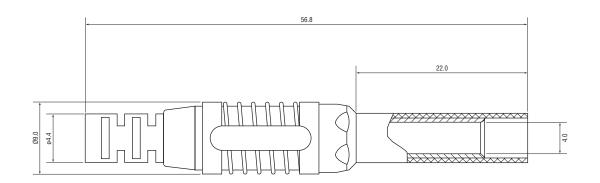
In-line 4mm safety socket accepting spring loaded 4mm plug, for self-assembly of test lead.
