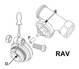
The RAVL adapter does not have to be screwed in place.
