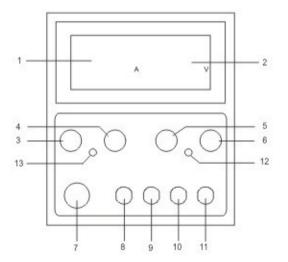
2.2.1 For constant voltage mode adjust controls 3 & 4 clockwise to the maximum position. Switch on the power ON/OFF switch 7 and adjust controls 5 & 6 to set the desired output voltage. Connect the load to the output terminals 8 & 10.
