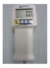
2. As soon as "0" is displayed, press "UNIT" button and "ZERO" button at the same time, until "CAL" appears on the display.
