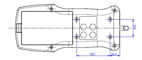
Mounting is possible on all SAUTER test stands by means of 4 x M3 screws.
