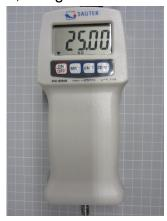
4. Put the corresponding weight at the loading hook. Avoid trembling and **keep still** while holding the weight. Hint: hold device with both hands while shoring up your elbows on a table or desk or fix it at a solid object (test stand).
