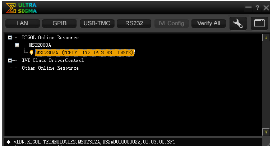
Figure 16-3 View the Device Resource under Control via LAN
