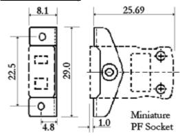
Recommended aperture size and hole pitch for panel mounting
