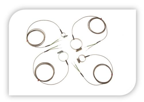
For pipe temperature measurement up to 350°C. They are available in a number of sizes to suit your diameter of pipe. These sensors make direct contact with the pipe for maximum performance and have grounded tips for a fast response.
