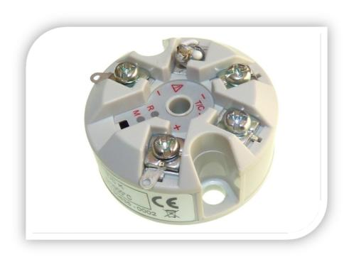
The push button temperature transmitter is a cost effective "smart" in head transmitter that accepts thermocouple temperature sensors and converts sensor output over a configured range to a standard industrial (4 to 20) mA transmission signal. A simple push button operation allows the user to select TC type, Burnout direction, Select fixed ranges and trim 4 and 20 mA points.
