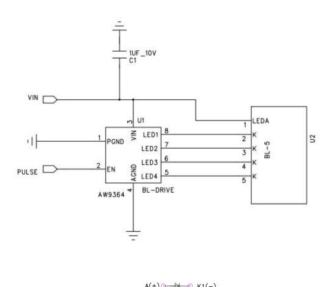
Note: constant current circuit for every LED, and though LED lamp current is less than 20mA.Recommand between 15mA and 20 mA for every LED.
