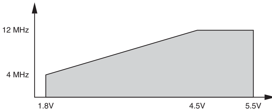
Figure 21-1. Maximum Frequency vs. V_{CC}
