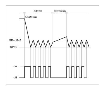
C02 - turn ON time delay for the compressor
