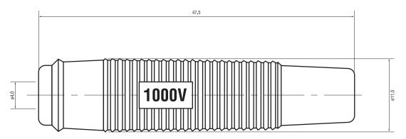
4mm Socket accepting spring loaded 4mm plug, especially used in automotive test accessories.
