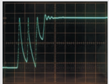
Arbitrary waveform - simulated contact bounce.
