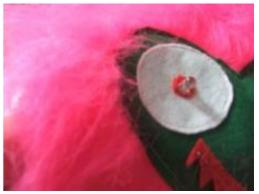
Taking one of the leds, push the metal legs through from front to back, leaving the domed part of the led on the front of the fabric and the legs on the
