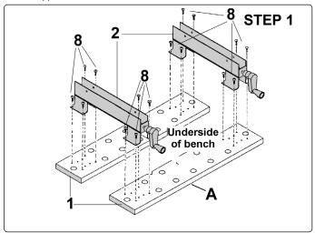
Lay the wooden worktop/jaws (1) upside down on a surface that will not scratch or cause damage. Screw the vice arms (2) to the jaws using wood screws (8) ensuring that the jaw angle and ruler guides are on the same side as the vice handles at point "A". **Note:** If not already assembled, push handles onto vice screw ends and secure with pins.
