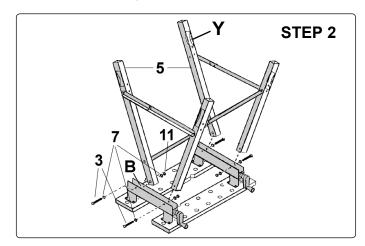
Open the leg frames (5) and align with holes on the inside of the vice arms at points "B" ensuring the curvatures on the lower part of the legs "Y" point outward. Insert bolts (3) from the outside of the vice arm with washers (7) and secure with washers (7) and nuts (11) from the inside.
