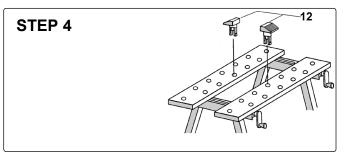
Fix chock (12) in suitable holes located in worktop as required.
