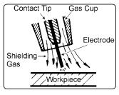
over the contact tip to direct the gas flow towards the weld ensuring that the arc welding process is shielded from oxidising air contaminates. The shielding gas also assists heating of the weld materials. The torch is connected to the positive side of a DC rectifier, and the negative clamp is attached to the workpiece.
