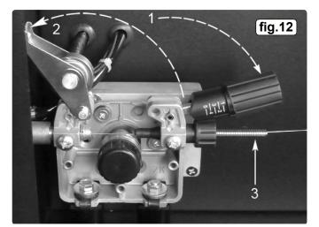
4.9.6 Set the wire speed knob to position 5 or 6. Keep the torch cable as straight as possible and press the torch switch. The wire will feed through the torch.
