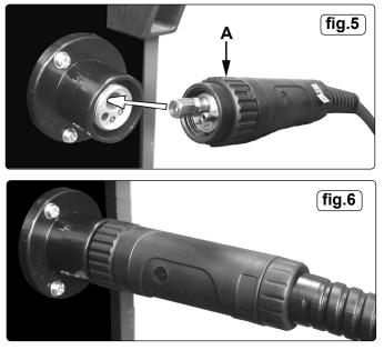
4.6. CONNECT THE TORCH CABLE TO THE WELDER. Align the pins on the Euro connector with the socket on the welder front panel as shown in fig.5. Push the connector into the socket and rotate the locking ring (A) clockwise so that it draws the plug into the socket as shown in fig.6.
