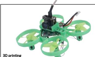
Entirely 3D printed using two separate parts. The main frame has the motor mounts, propeller ducts and flight controller mounts. The camera is mounted using a separate bracket.
