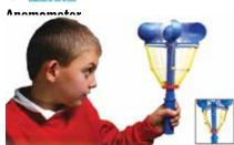
This unique design gives a direct reading of wind speed, without the need to count revolutions. The low and high calibrations register ms-1 and the Beaufort scale.
