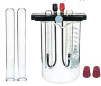
Brownlee's Water Electrolysis Apparatus is used to demonstrate that electrically conductive liquids can be decomposed and resolved into their constituent elements by means of a unidirectional electric current. The gaseous components formed by this method can be trapped and their relative volumes estimated.
