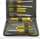
Kit contains: 3mm flat blade screwdriver No. 0 Phillips screwdriver Reversible T10 and T15 torx screwdriver Reversible No. 1 Phillips and 5mm flat screwdriver 1/4 and 3/16in. nut drivers
