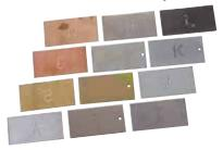
This 12-piece metal strip set includes a strip of each of aluminium, brass, copper, bronze, nickel, mild steel, galvanized iron, magnetic and non-magnetic stainless steel, zinc, chrome and lead.
