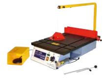
The C R Clarke 280 hot wire sculptor allows you to accurately cut thermoplastic foam into a wide range of shapes. Its adjustable guides accurately place the material and its wire bow protractor accurately sets angles to produce wedges, chamfers and cones.
