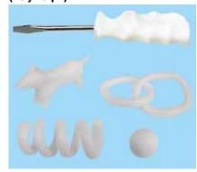
Polymorph is one of a new generation of polymers with all the characteristics of a tough, machinable engineering material, yet it fuses and becomes easily mouldable between 30°C and 62°C.
