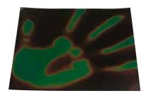
A self-adhesive 150 x 150mm sheet printed with a thermochromic liquid crystal ink which changes colour when heated above 27°C.
