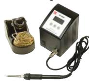
The LF-1600 soldering station has a digital temperature indicator, detachable 80W soldering iron and a Set-and-Forget temperature control to select a temperature between 200 and 480°C (392 to 896°F).
