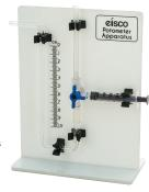
The apparatus is mounted on a strong backing plate and consists of a capillary tube with a millimetre scale, connected via a three-way tap to a syringe. A cut shoot is connected to third outlet.
