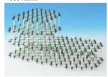
This skeletal Graphite model is particularly suitable for showing the nature of the solid as it is effectively transparent in depth.
