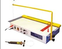
The Triform 180 from C R Clarke is a 3-in-1 machine that cuts and sculpts expanded thermoplastic material as well as bending thermoplastic sheet up to 6mm thick.
