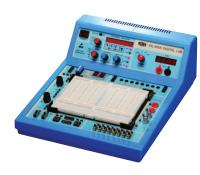
This comprehensive digital electronics training system contains a wealth of equipment and features. The training system contains all the peripherals needed to support your circuit design. Components can be connected without soldering, by simply inserting them into the breadboard. Your circuit can then be powered by the internal power supplies, signals applied from the function generator and monitored on the built-in test equipment and displays.
