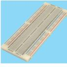
number of holes, 0.3 to 0.8mm wire size acceptability, 3A contact current, ABS polymer body material, silver nickel contact material, 4 rows of 50 interconnected sockets suitable for use as power supply rails, all contact positions are clearly defined on an alphanumeric grid.
