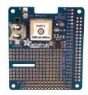
an external antenna. Additional features include status LEDs, PPS output on fix, and it is possible to obtain 7 years timekeeping by using a CR1220 backup battery (not supplied).
