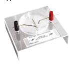
surface. Various electrode configurations can be arranged in the liquid and when a high voltage is applied via the 4mm terminals the field pattern is generated. The see-through base allows the pattern to be projected via an overhead projector system.
