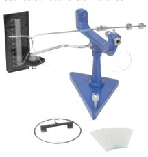
This Searles Surface Tension Balance can be used to demonstrate the surface tension of a liquid by allowing it to be shown on a graduated scale.
