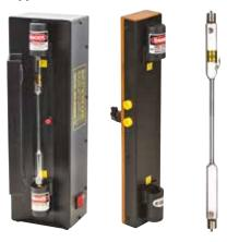
A range of spectrum tubes, associated holders and power supplies, for use in spectral analysis experiments.
