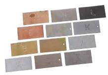
This 12-piece metal strip set includes a strip of each of aluminium, brass, copper, bronze, nickel, mild steel, galvanized iron, magnetic and non-magnetic stainless steel, zinc, chrome and lead.
