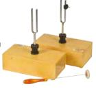
One fork is provided with an adjustable mass, by means of which the frequency of that fork may be shifted from the nominal 440Hz. When both forks are sounded at the same time, a clearly audible 'beat' is produced, its rate depending upon the difference in frequency between the two forks.
