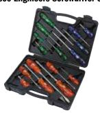
Expert Quality , professional screwdrivers have chrome vanadium steel blades hardened, tempered with satin chrome plated finish and sand blasted tips. The generous size handle is manufactured from high quality transparent PVC. Colour coded handles for easy recognition. Some blades have hexagon bolsters which enable extra power to be applied by use of an open end spanner. Packed in blow mould case with sleeve.
