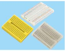
A range of Solderless Breadboards that allow components to be easily connected together into circuits and can be used again and again for experiments and prototyping.
