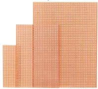
This stripboard provides a simple form of printed circuit, ideal for prototype and development work. The board has holes and strips on a 2.54mm pitch and is manufactured from copper-clad paper and phenolic laminate body material
