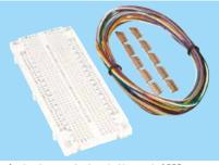
Professional prototyping board with a total of 555 contacts arranged in two blocks of 43 rows of five interconnected sockets on a 2.54mm (0.1in) pitch.
