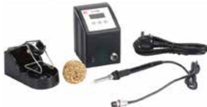
The Xytronic LF-1700, 100W Digital Soldering Station has a digital temperature readout and a soldering temperature range of 150 to 480°C. Its electronic circuitry maintains the soldering temperature by means of a temperature sensor mounted in the soldering iron. The electronic circuitry employs Zero Voltage switching techniques that prevent the generation of voltage and current spikes that could damage sensitive components.
