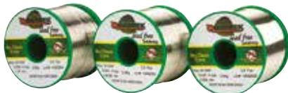
A flux-cored solder wire made from SAC305 (965-30), a lead-free alloy consisting of 96.5% tin, 3% silver and 0.5% copper. The NC601E flux is a colophony-free, no-clean type that leaves virtually no post-soldering residue for a visibly clean solder connection.
