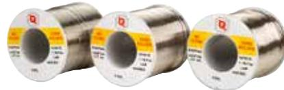
A flux-cored solder wire made from an alloy consisting of 60% tin and 40% lead. The NC601E flux is a colophony-free, no-clean type that leaves virtually no post-soldering residue for a visibly clean solder connection.
