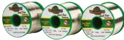
A flux-cored solder wire made from SN100e, a lead-free alloy consisting of 99.5% tin, 0.5% copper and a trace of cobalt. The NC601E flux is a colophony-free, no-clean type that leaves virtually no post-soldering residue for a visibly clean solder connection.
